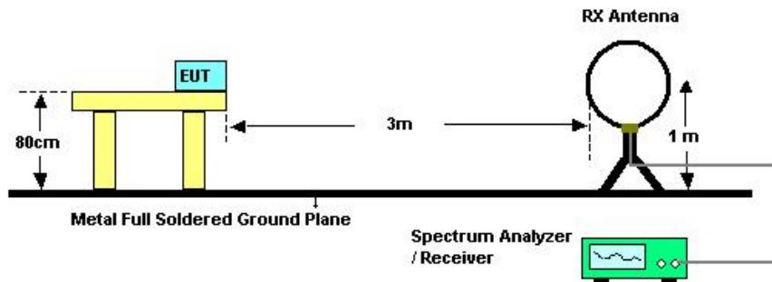
For Radiated Emissions: 30MHz~1GHz
