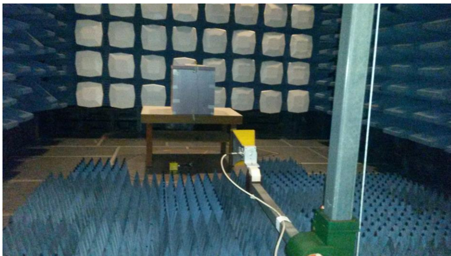
Radiated Emissions Setup in Semi-Anechoic Chamber, 1GHz-18GHz
