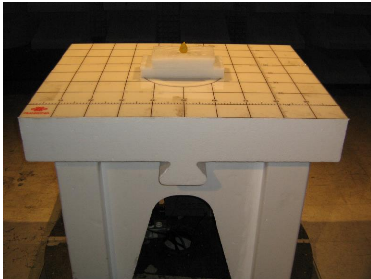
Radiated Emissions Setup in Semi-Anechoic Chamber, 30MHz-1GHz
