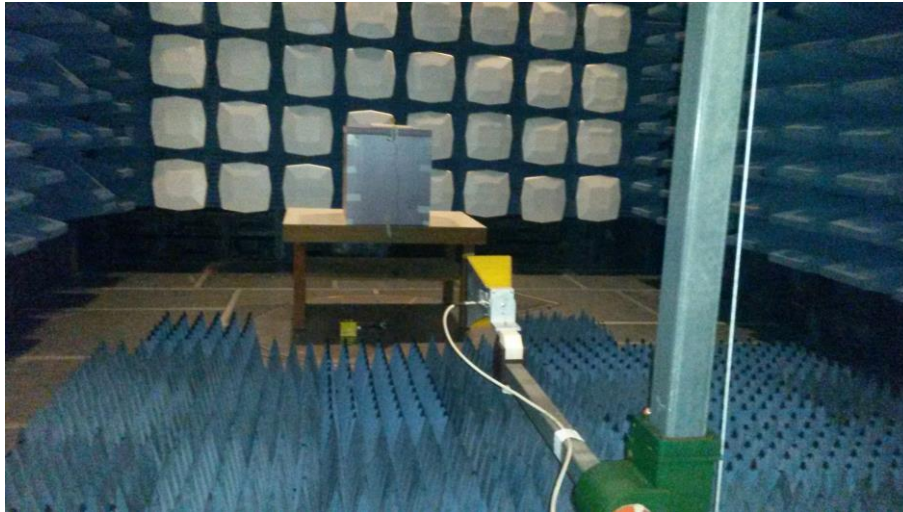
Radiated Emissions Setup in Semi-Anechoic Chamber, Above 1GHz
