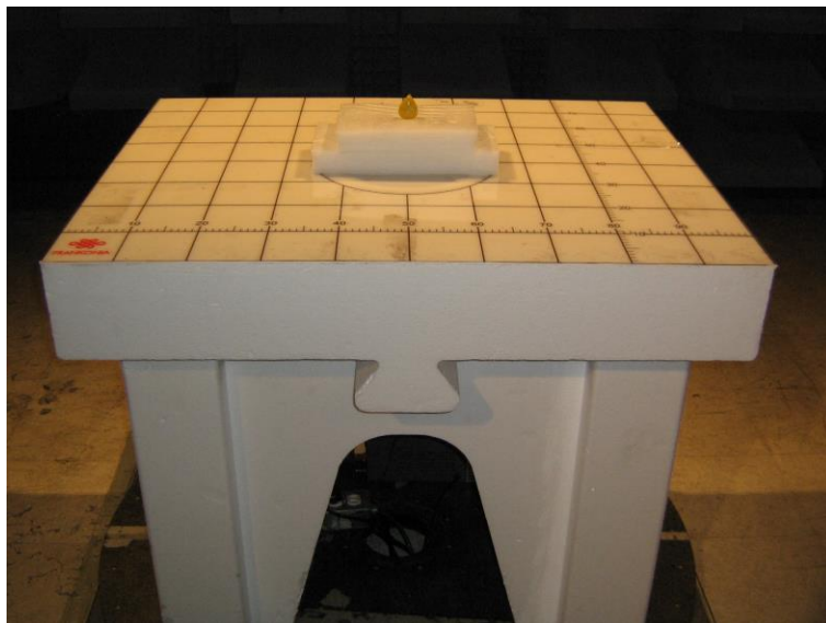
Radiated Emissions Setup in Semi-Anechoic Chamber, 30MHz-1GHz
