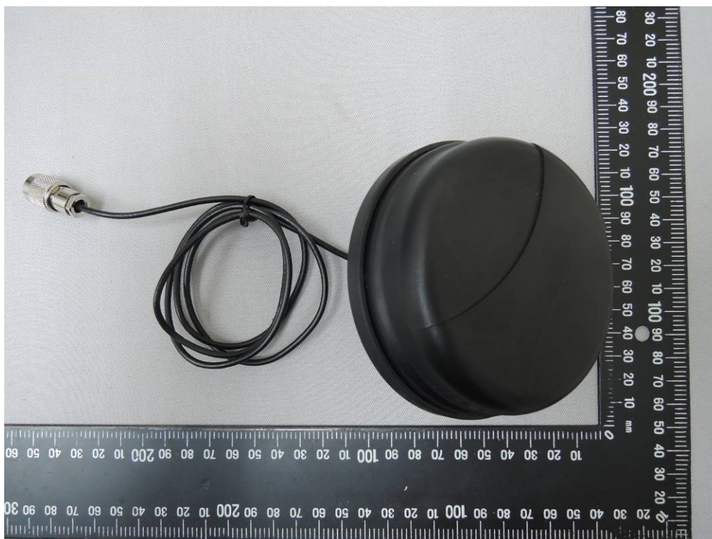
WWAN Antenna-2 (Model No.: MHD1891, Supplier: Badland)
