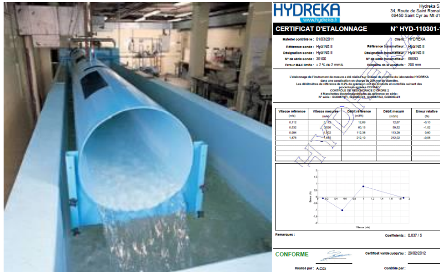
Figure 42: Hydraulic bench for the calibration of HydrINS 2 / HydrINS 2 Mini flow meters and HYDREKA calibration certificate
