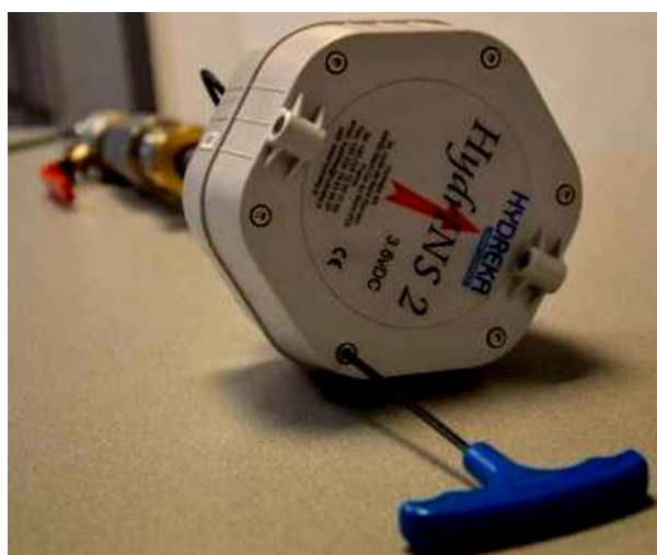
Figure 23: Remove the screws from the head of the HydrINS 2 flow meter
