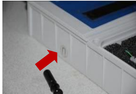
Figure 21: Application of the magnet to the magnetic switch to activate the Display
