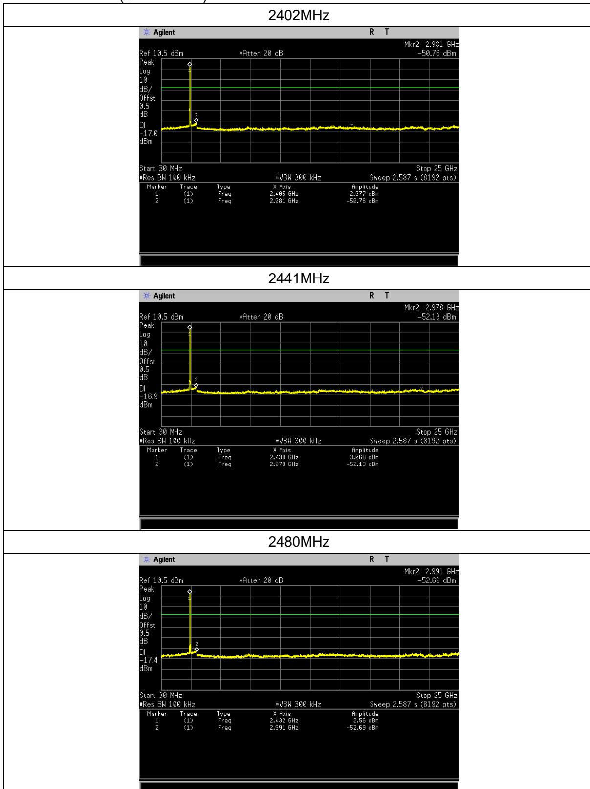
Conducted emission ( $\pi/4$ -DQPSK mode)
