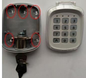
3. Locate the base where needs to install, mark the 5 opened holes in order to fix them.
