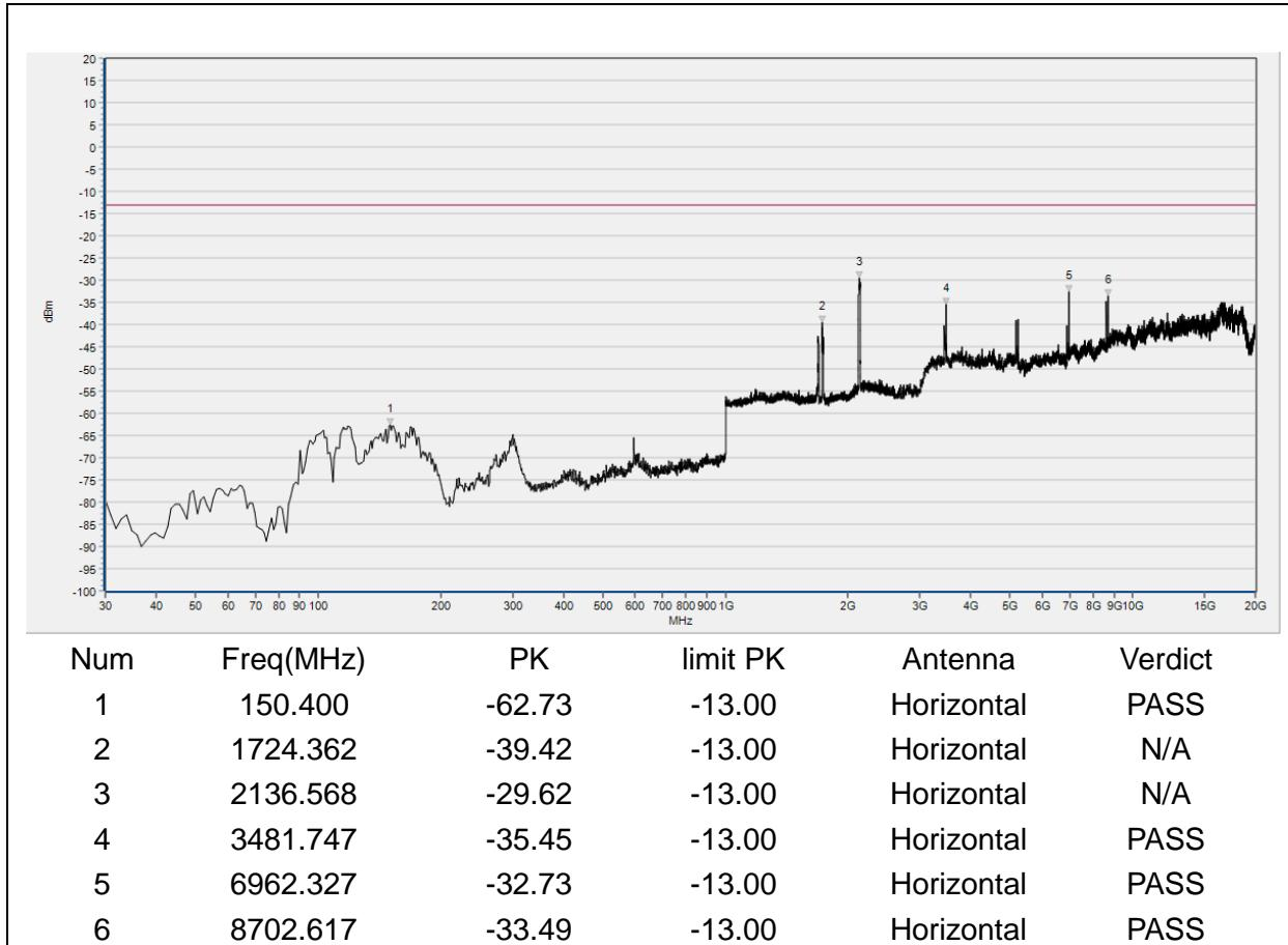
(LTE Band4, 20MHz BW, QPSK, Mid Channel, Horizontal)
