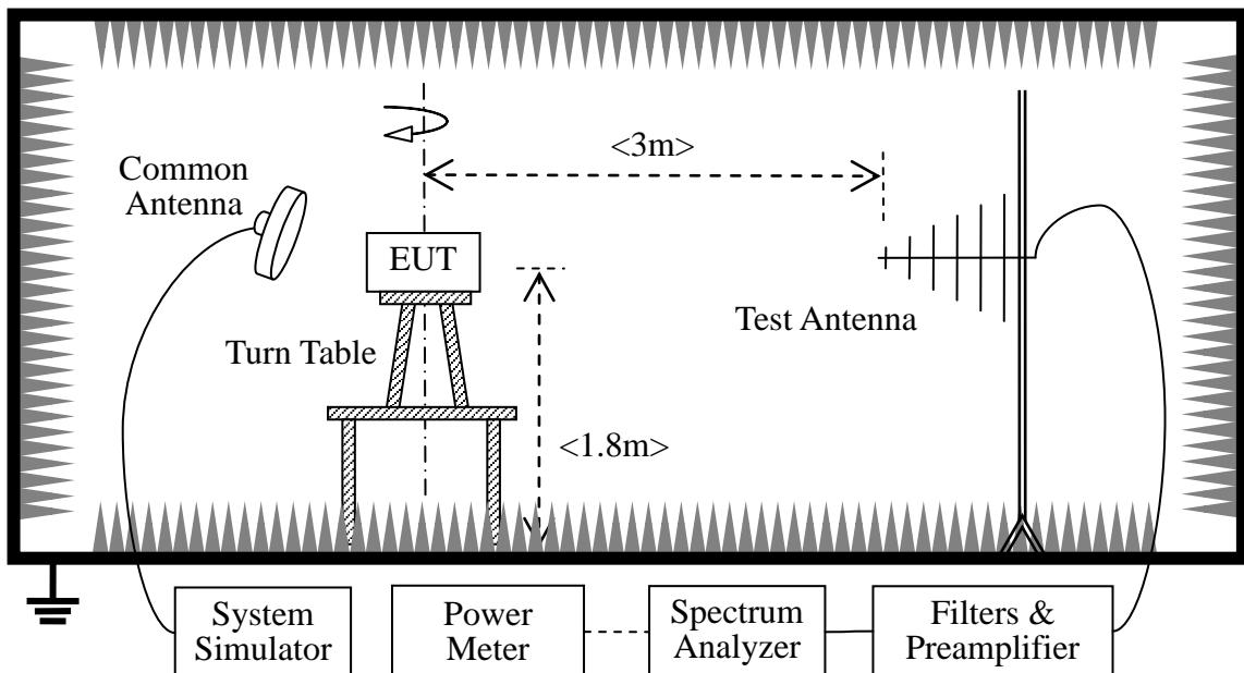
The EUT, which is powered by the PC, is located in a 3m Full-Anechoic Chamber; the cable loss, air loss and so on of the site as factors are pre-calibrated using the "Substitution" method, and calculated to correct the reading.
