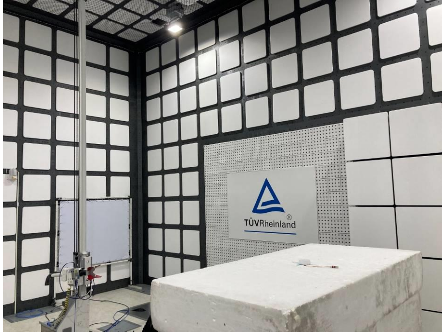
Photograph 5: Test Setup for Spurious Emissions (Back View 3)
