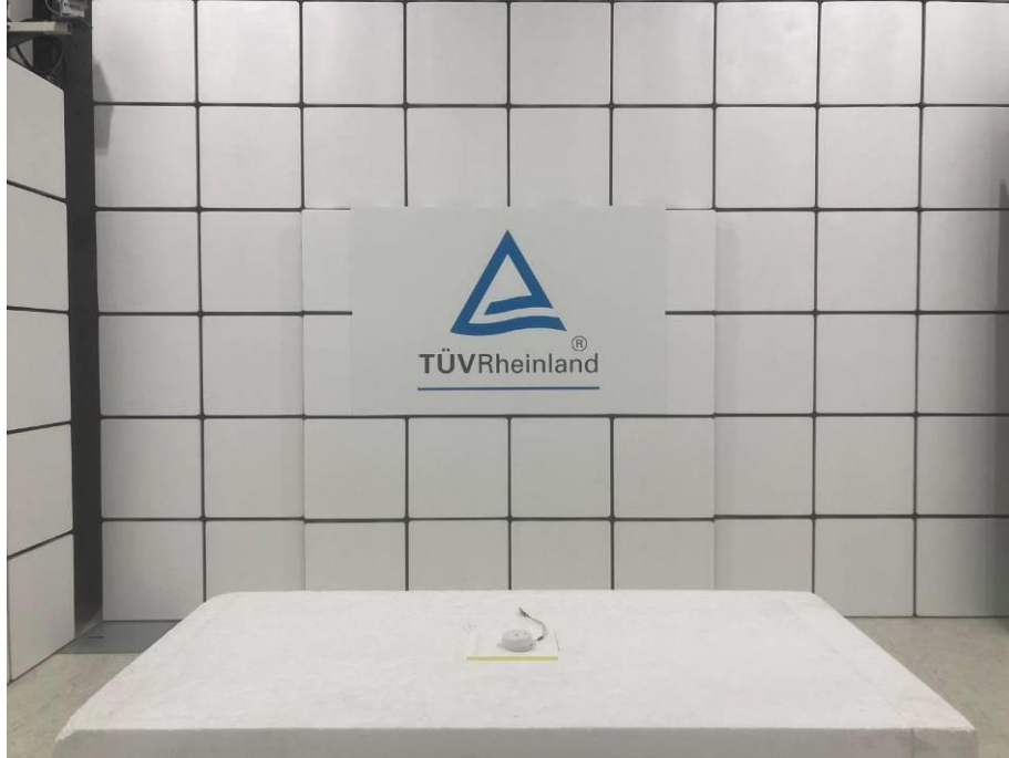
Photograph 1: Test Setup for Spurious Emissions (Front View 1)
