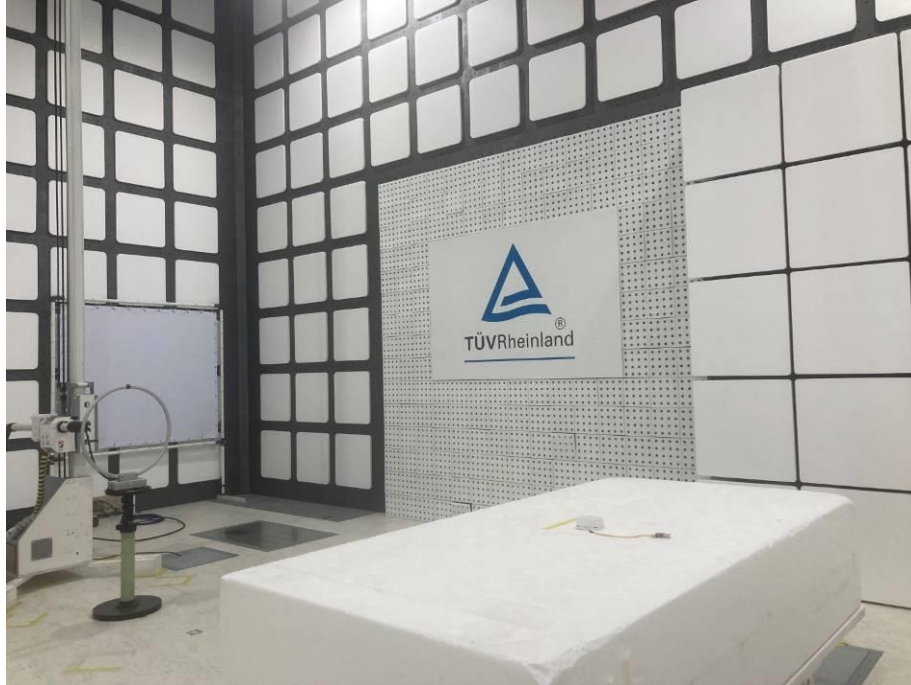
Photograph 3: Test Setup for Spurious Emissions (Back View 1)
