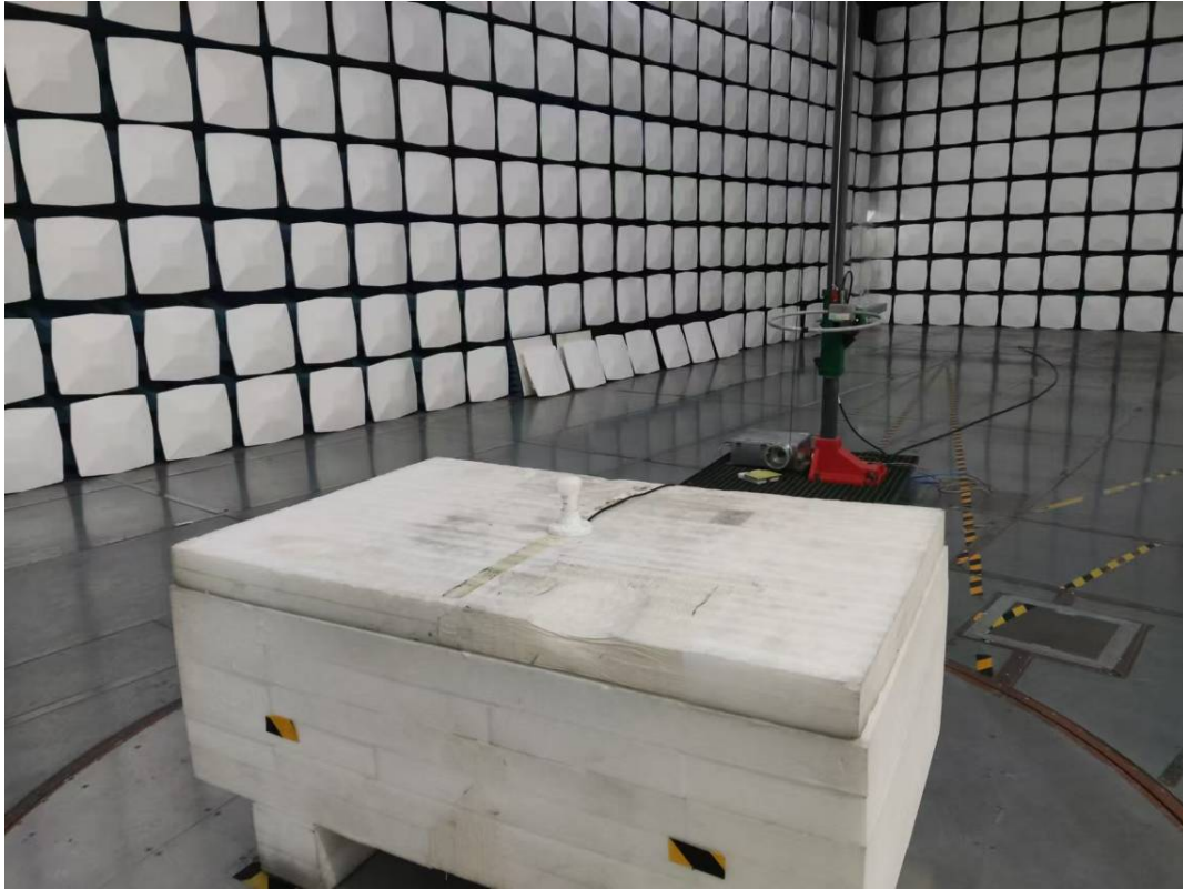
Radiated Emission 30M-1GHz View
