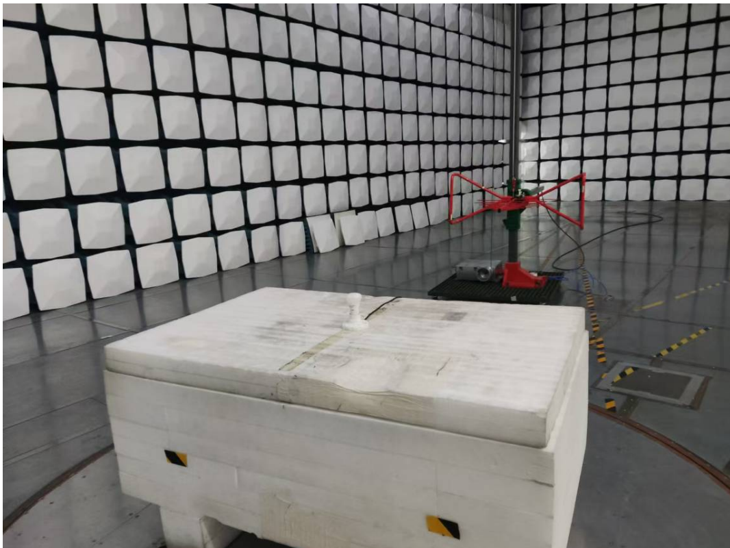
Radiated Emission 30M-1GHz View
