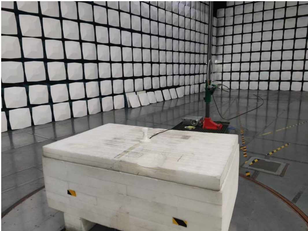
Radiated Emission 9k-30MHz Perpendicular View
