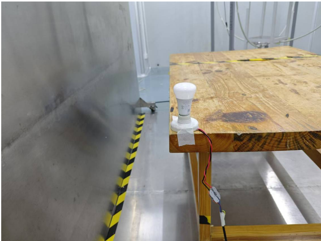
Conducted Emissions Side View
