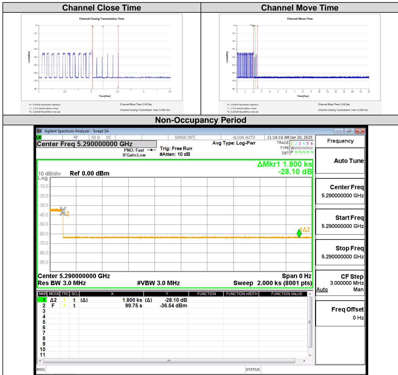
**Band 3****IEEE 802.11ac VHT80 mode / 5530 MHz****Type 0 Channel Move Time Results & Channel Closing Transmission Time Results**
