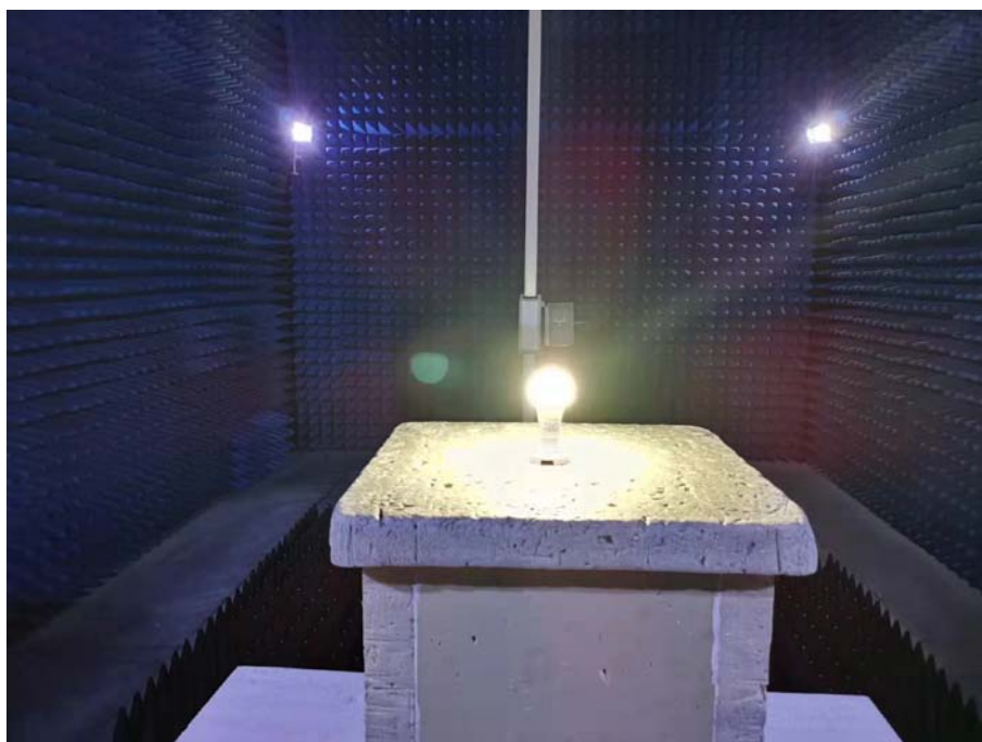
Photo of Radiated Emission Measurement Above 1GHz
