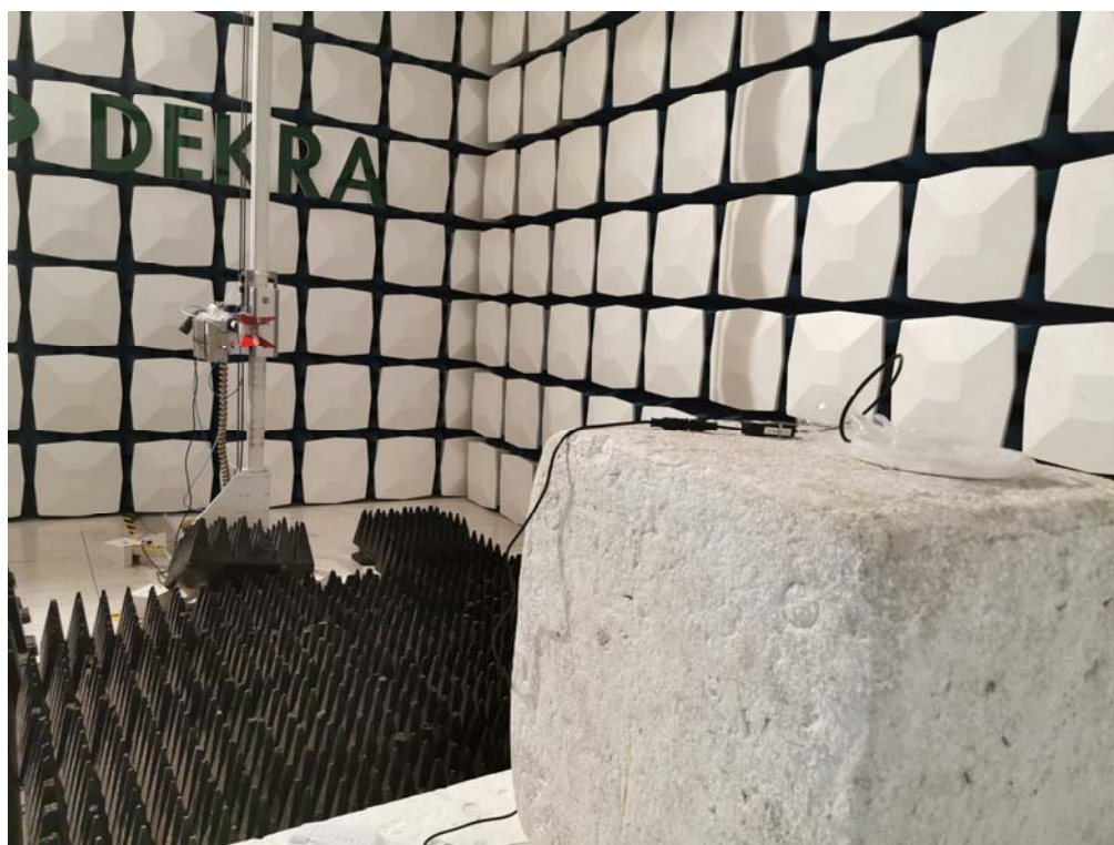
Description: Radiated Emission Test Setup for 1~18GHz
