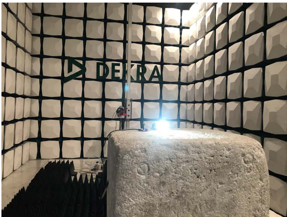
Description: Radiated Emission Test Setup for 1~18GHz
