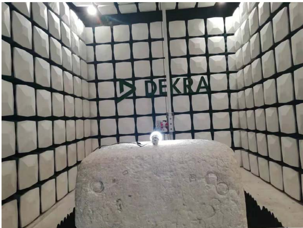
Description: Radiated Emission Test Setup for 1~18GHz
