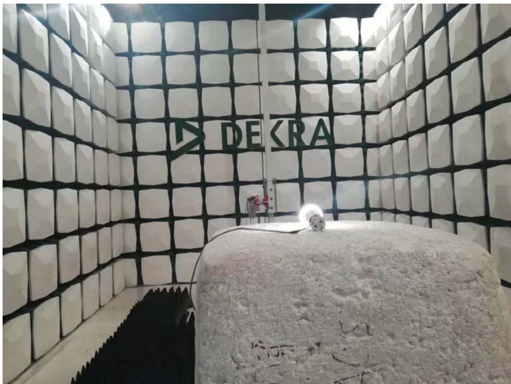
Description: Radiated Emission Test Setup for 1~18GHz
