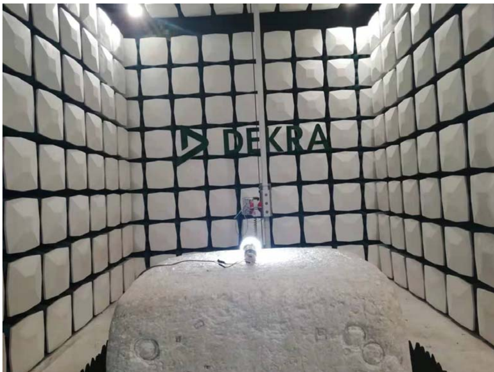
Description: Radiated Emission Test Setup for 1~18GHz
