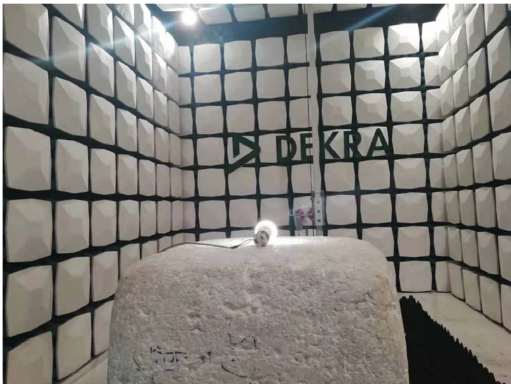
Description: Radiated Emission Test Setup for 1~18GHz
