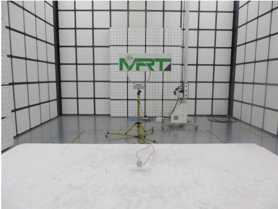
Radiated Emission Setup 9k~30MHz
