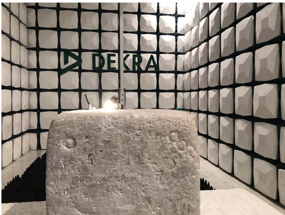
Description: Radiated Emission Test Setup for 1~18GHz
