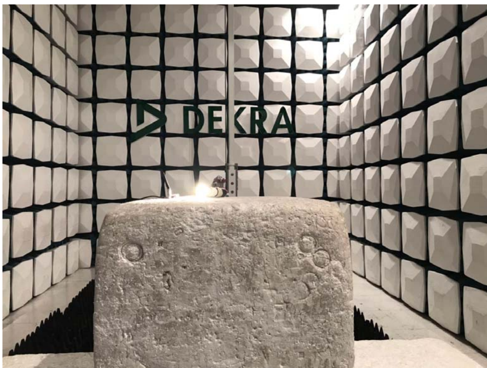
Description: Radiated Emission Test Setup for 1~18GHz
