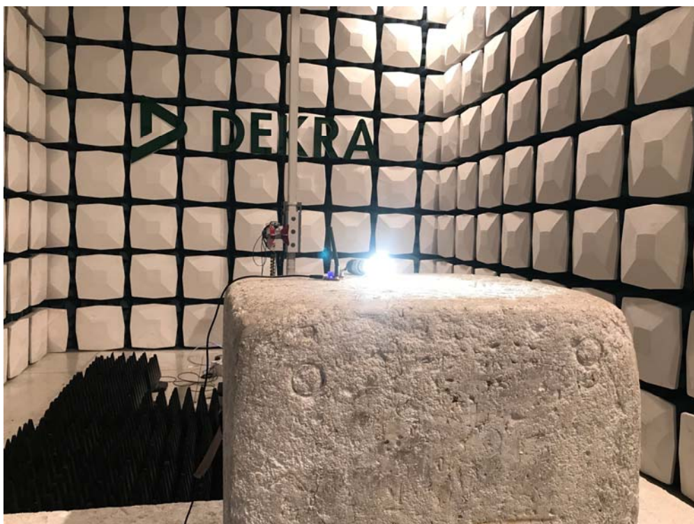
Description: Radiated Emission Test Setup for 1~18GHz
