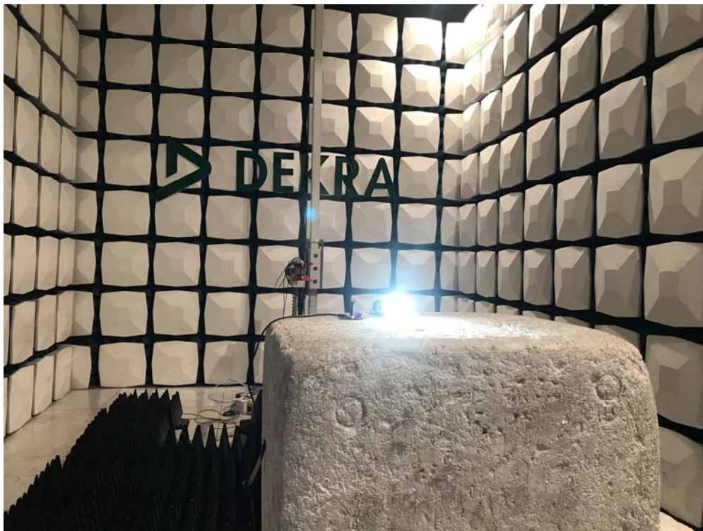
Description: Radiated Emission Test Setup for 1~18GHz
