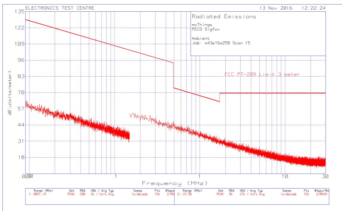
**Plot of Test Chamber Ambient: (measurement noise floor):**
