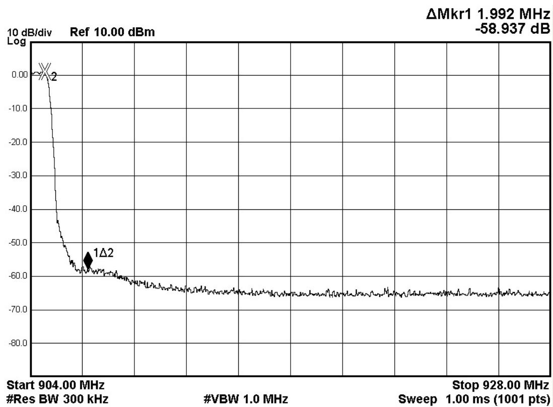
Screen Capture from the spectrum analyzer: Upper Band Edge, non-hopping
