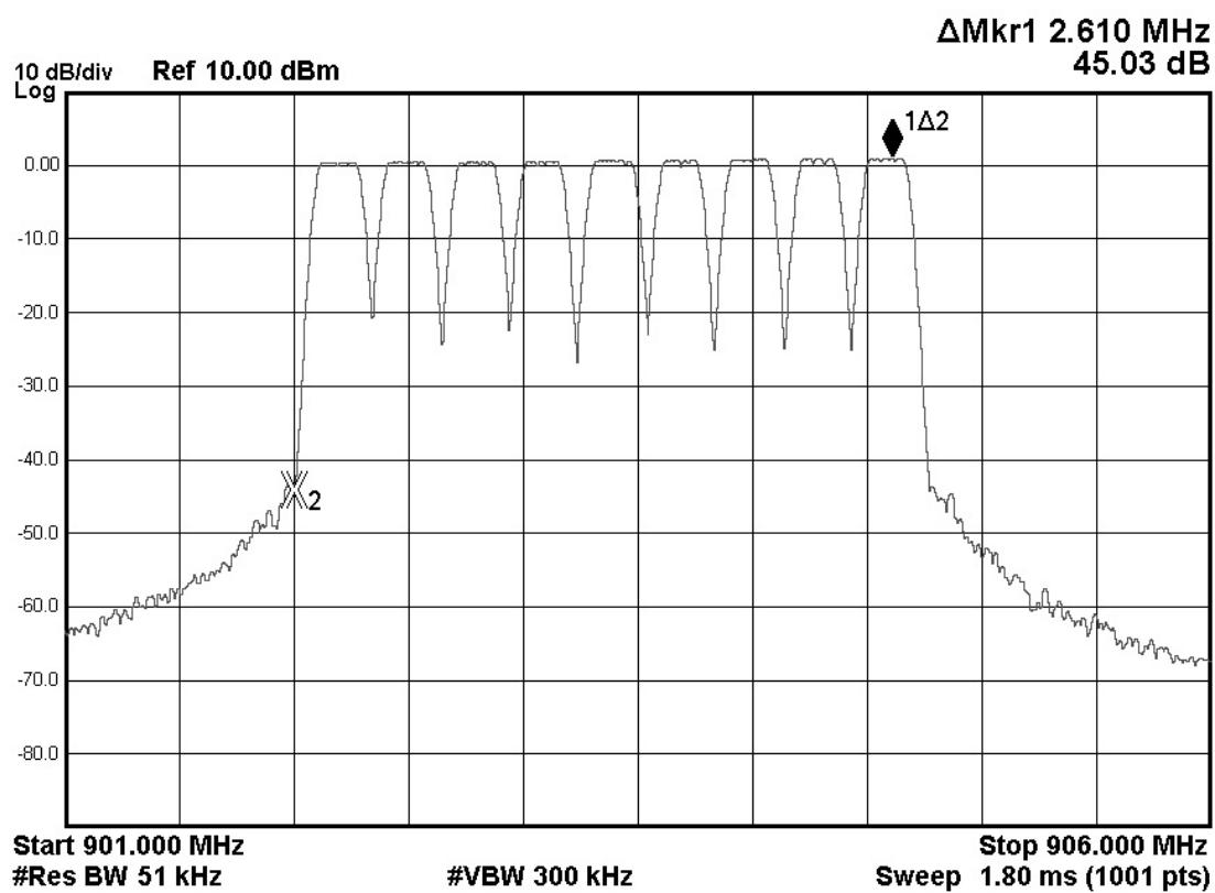
Screen Capture from the spectrum analyzer: Lower Band Edge, non-hopping
