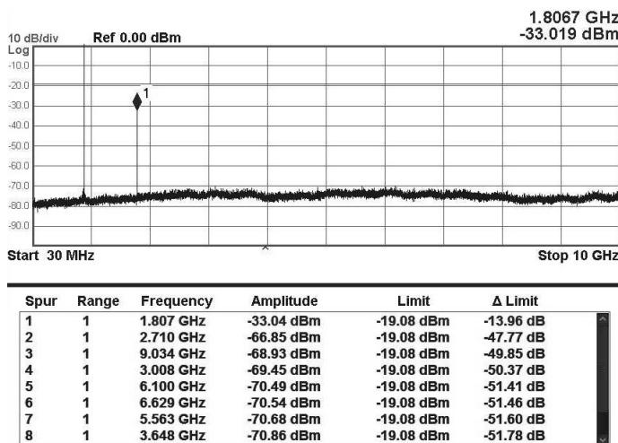
Screen Capture from the spectrum analyzer: High  $f_c$
