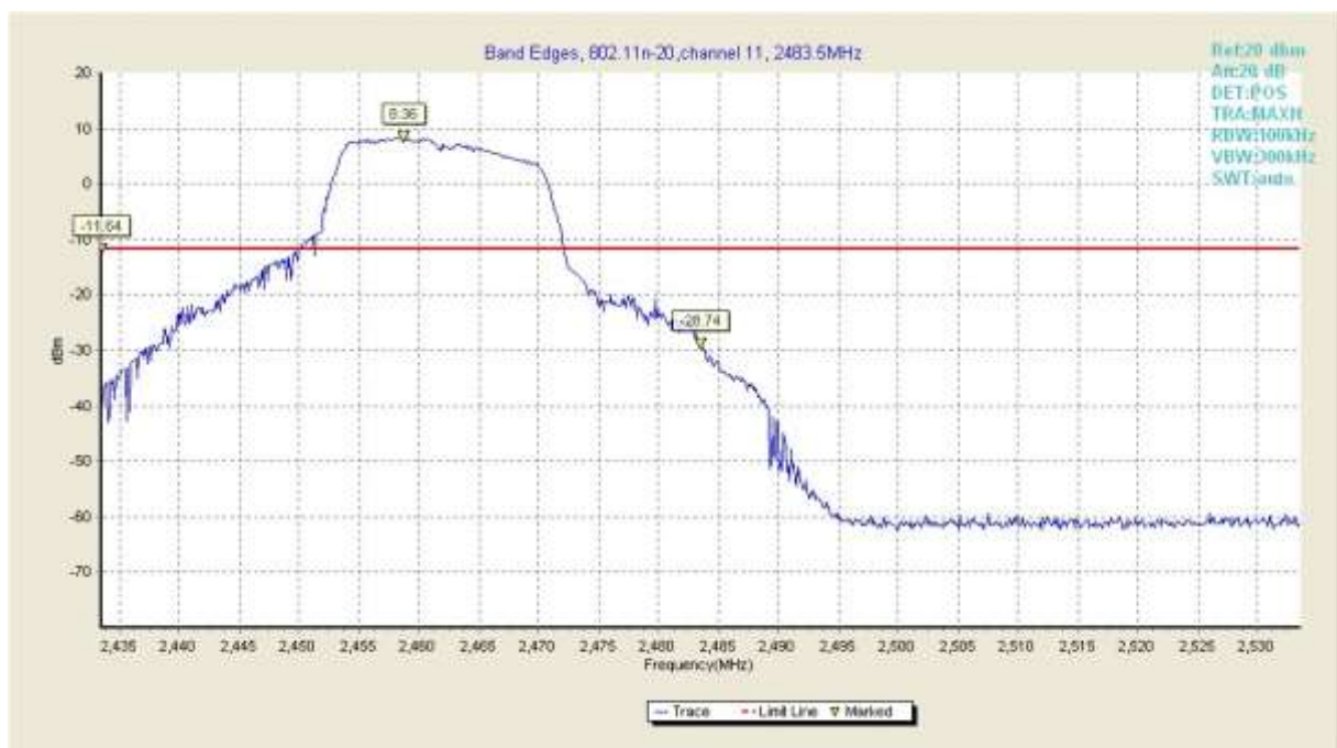
Fig30. Frequency Band Edges of 802.11n-20 in channel 11,2483.5MHz
