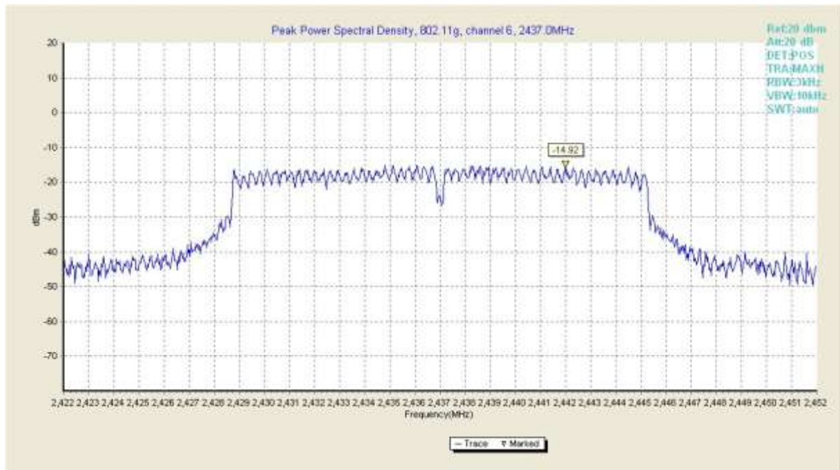
Fig.5 Peak power spectral density of 802.11g in channel 6,2437MHz
