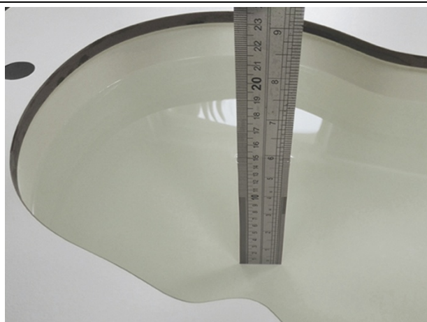
Liquid depth in the head phantom (2450MHz)
