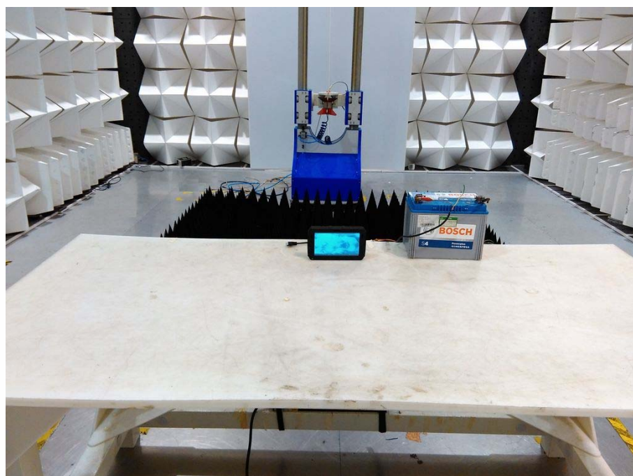
Radiated spurious emission Test Setup-2 (Above 1GHz)
