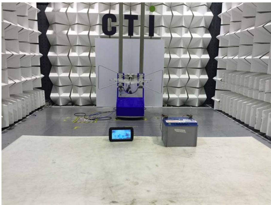
Radiated spurious emission Test Setup-1 (Below 1GHz)
