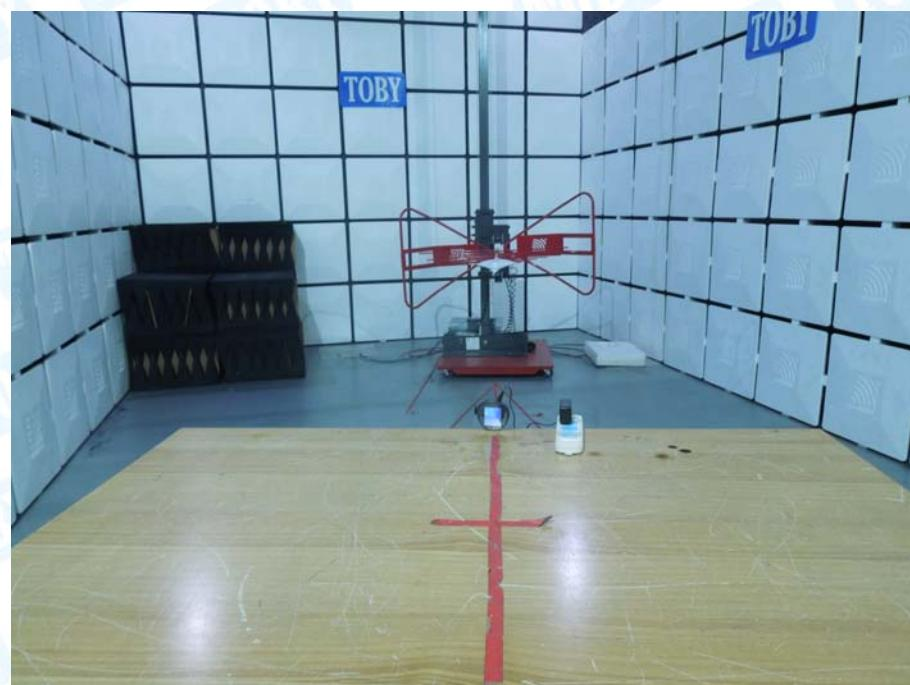
**Photo of Setup for Conducted Emission**
