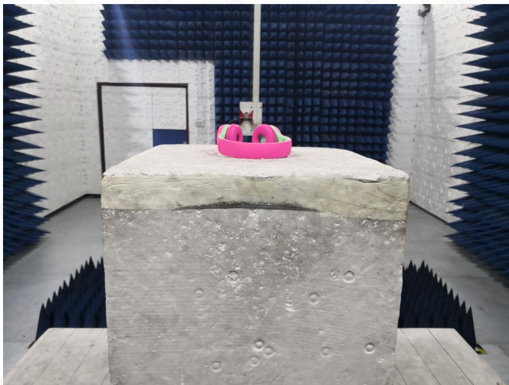
RADIATED EMISSION TEST SETUP ABOVE 1GHZ
