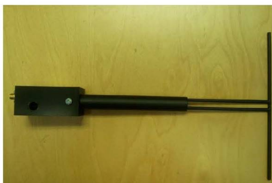
Figure 1 – MVG COMOSAR Validation Dipole
