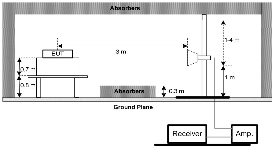
(C) For radiated emissions below 30MHz
