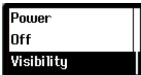
**(1) Bluetooth settings**: 1) Press the Enter key can be turned on or off Bluetooth, BT watch Bluetooth turned off by default, Bluetooth is turned on if the status bar of the main menu screen will display a small icon "X";
