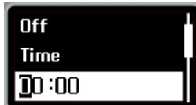
2)、Set the time : Press the switch button to jump to different locations numeric setting, each location can press the volume keys up or down to adjust the specific numbers, setup is complete press OK to save the settings.
