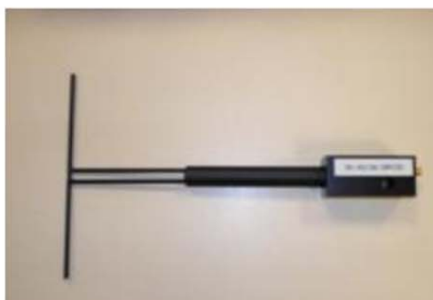
Figure 1 – Satimo COMOSAR Validation Dipole
