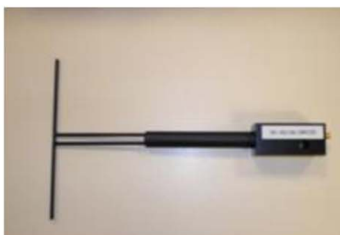
Figure 1 – Satimo COMOSAR Validation Dipole
