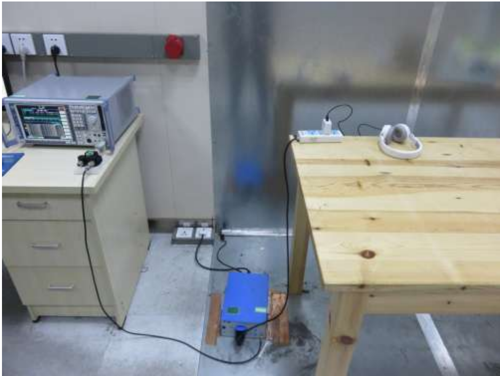
FCC RADIATED EMISSION TEST SETUP
