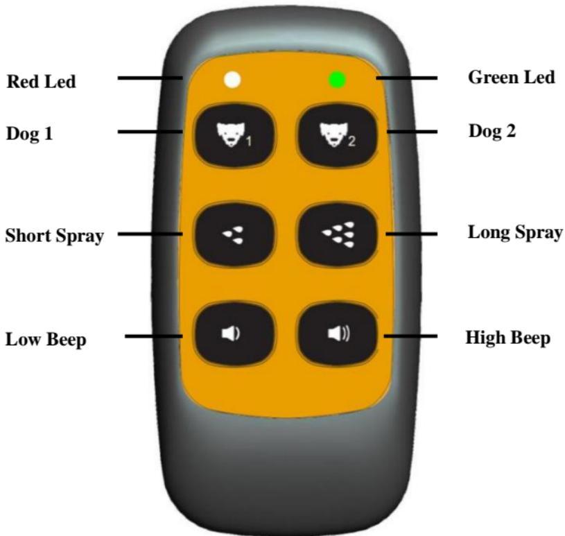
**Red Led:** Indicates the first dog and low battery. Press the Dog1button or Spray button or beep button one time, the Red led light will flash one
