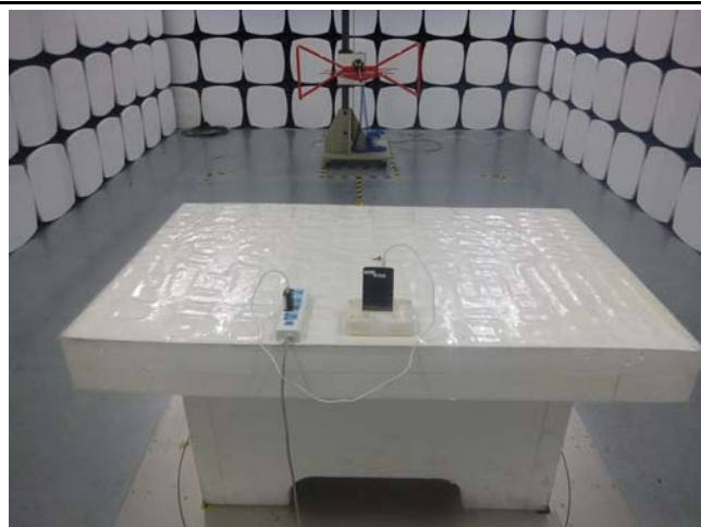
Conducted Emissions Test Setup Front View
