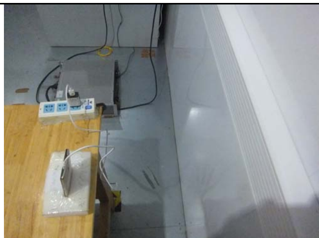
Conducted Emissions Test Setup Side View
