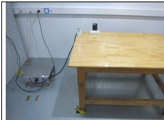
Conducted Emissions Test Setup Front View
