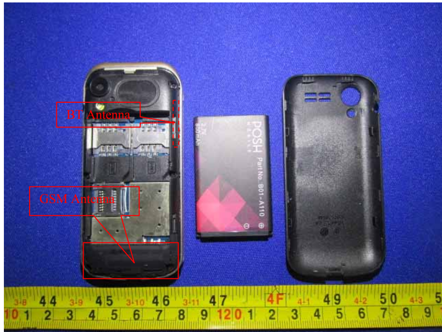
EUT – Cover off View
