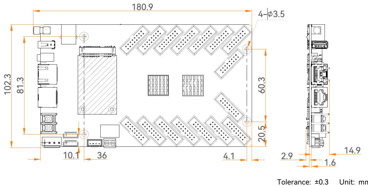
To make molds or trepan mounting holes, please contact NovaStar for a higher-precision structural drawing.
