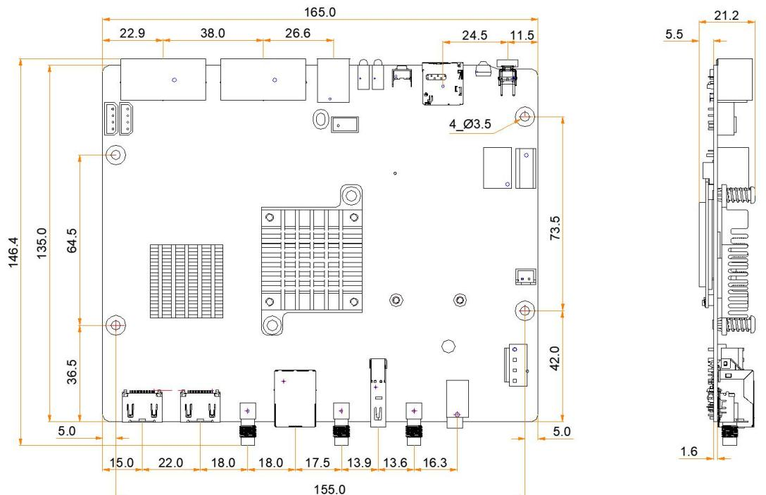
Tolerance:  $\pm 0.3$  Unit: mm
