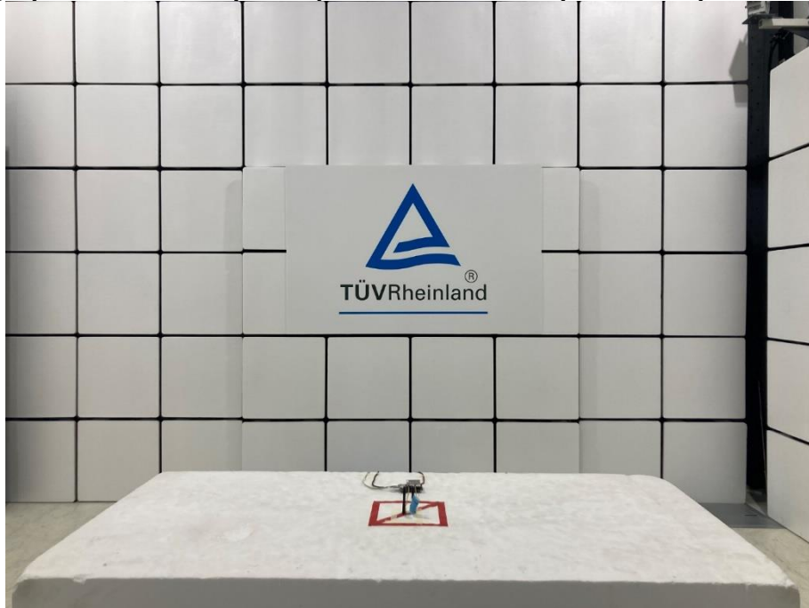
Photograph 10: Test Setup for Spurious Emissions (Front View)
