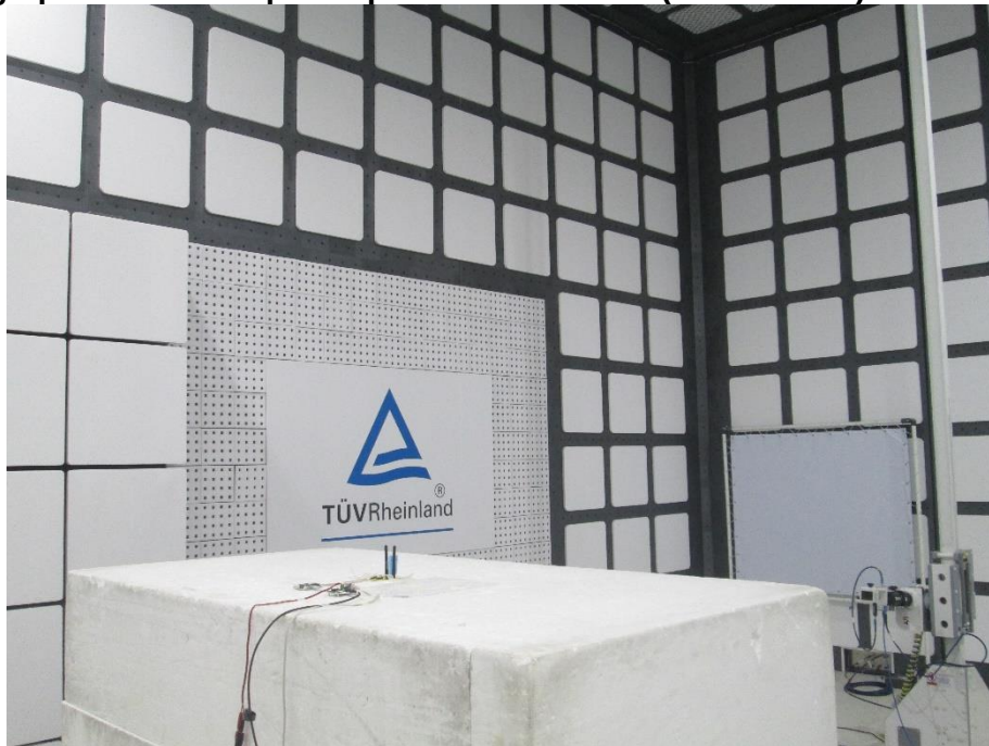
Photograph 6: Test Setup for Spurious Emissions (Back View 4)
