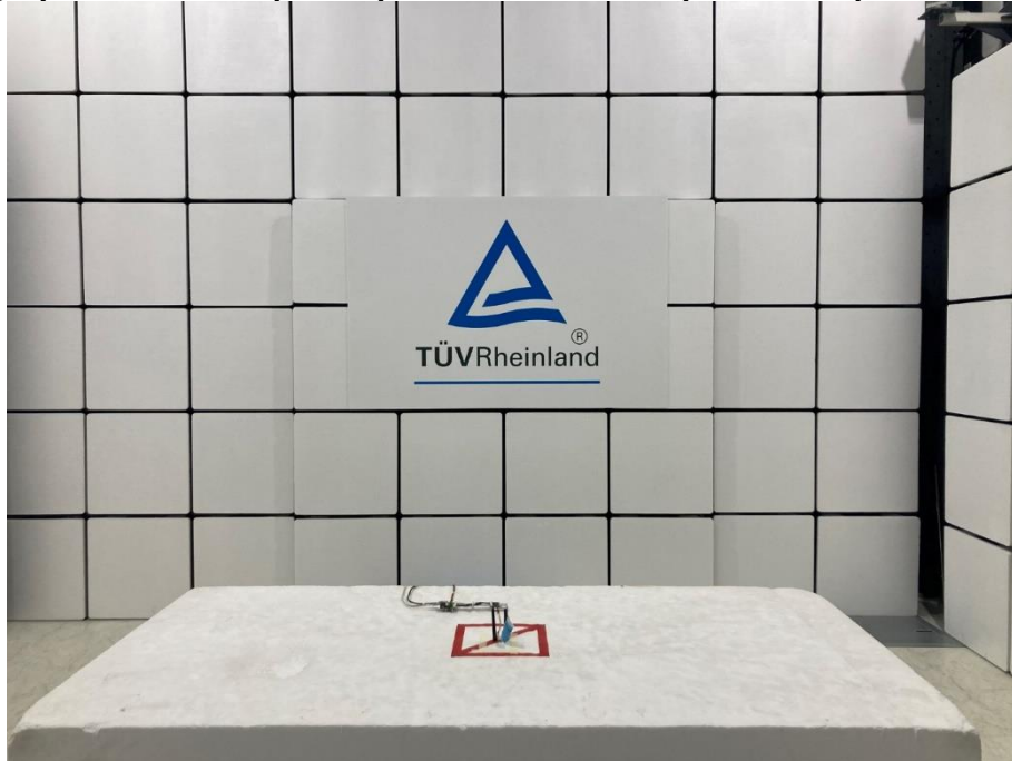
Photograph 7: Test Setup for Spurious Emissions (Front View)
