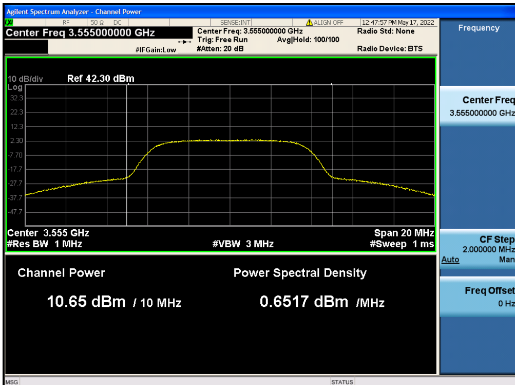
RF measurement plot for WINNF.PT.C.HBT.1 Test Case ID_BW10M_Grant maxEirp 23_Ant.2
