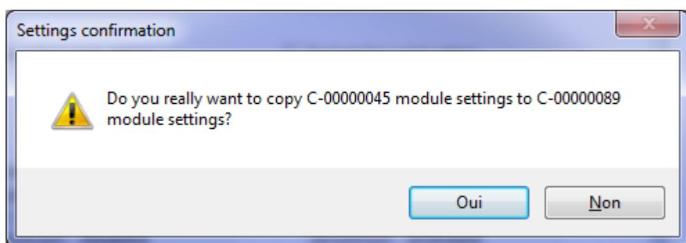
By clicking « **Yes** », the configuration is copied from module **C-00000045** to module **C-00000089**.
