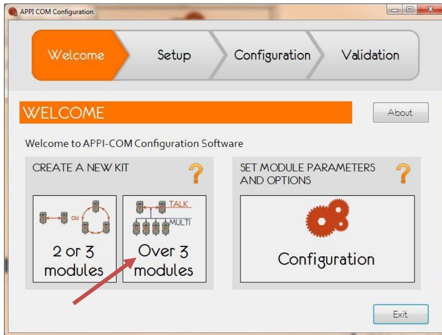
3. After clicking "More than 3 modules", the software requests to connect the modules and displays the number of recognized ones:
