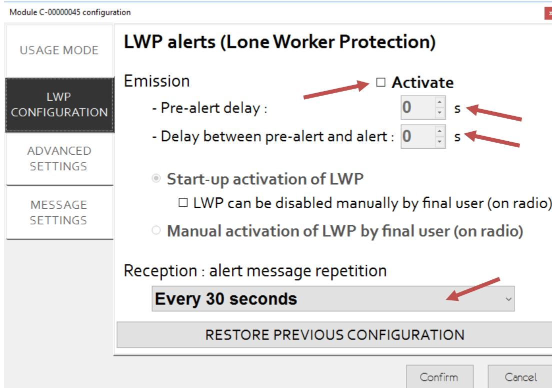
This window allows activate the LWP function and set the parameters up:
