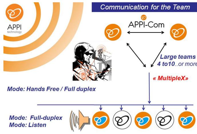
It can be useful that "**Multiplex**" module are connected to an Audio headset through a PTT, so that it does not permanently occupy the third slot and prevent the other multiplex modules to intervene in the conversation. Alternatively, they are using the "VOX" mode (see later one) to prevent non desired communication and maintain the communication fluidity.
