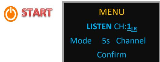
The proposed channel ("CH 1<sub>LR</sub>" in the example) is the last channel in use. The user can, for 5 seconds (countdown), change the channel using the keypad:
