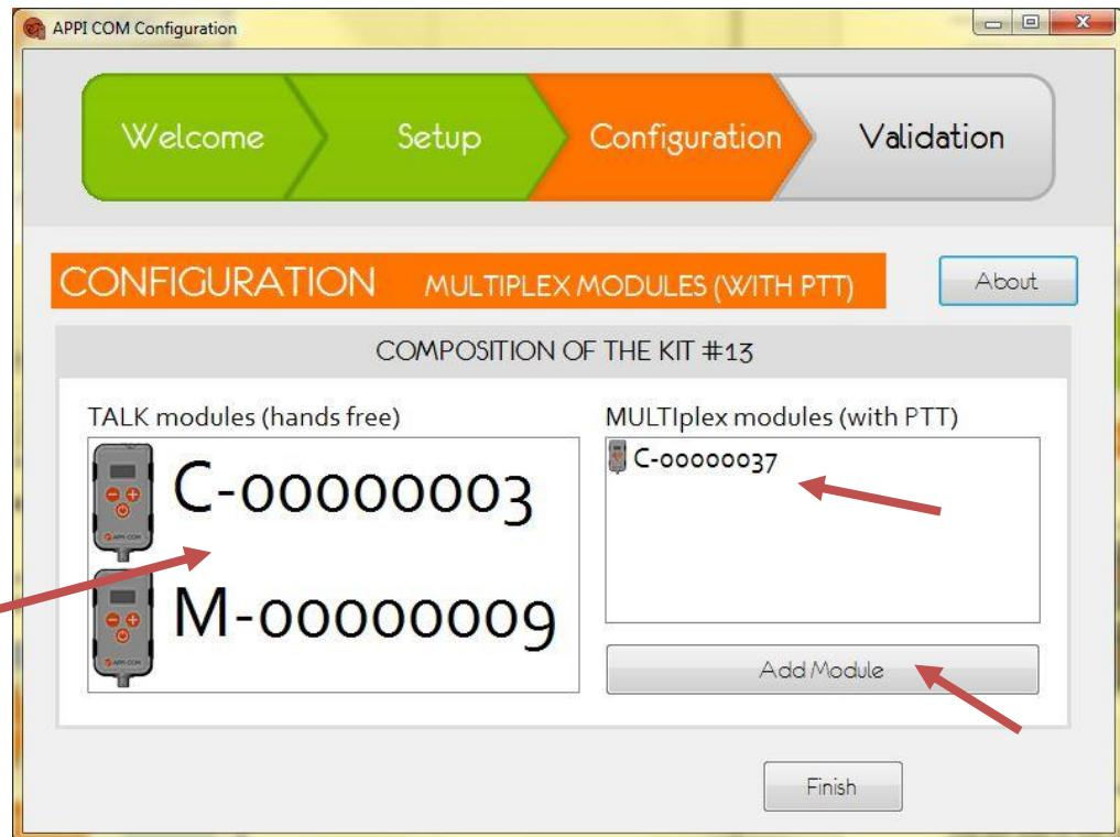
The left side of the window shows the ID of the two “Talk” modules, while the left side zone displays all the “**Multiplex**” modules added to the kit.
