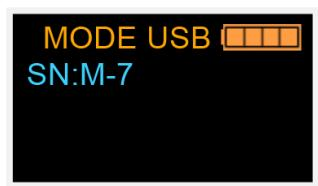
⇒ To reinstate the "communication" mode, disconnect the USB cable and turn the module on.
