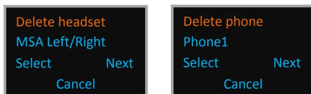
The menu propose to delete the first device paired, its name is printed on the second line.
