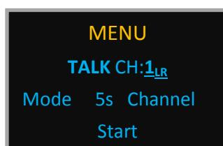
**Note:** **Long Range** Channels are noted « 1\_LR, 2\_LR, etc. » while the **Short Range** ones are labelled "16sR" (example)
