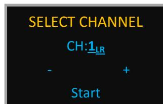
With this menu, one can select one of the 19 channels (1 à 19) with the and keys. When the desired channel is displayed, press to validate and start communicate.
