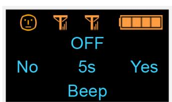
If the user takes no action, the shutdown procedure is canceled after 5 seconds and the system goes back to the main screen.
