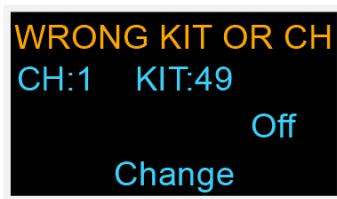
The "**WRONG KIT OR CH**" message blinks and the screen displays the selected Kit and Channel Numbers (Channel **1** and Kit **49** in this example). The user then would:
