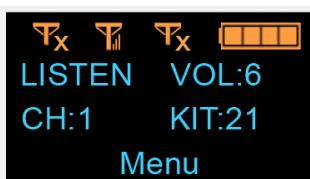
**EXAMPLE 2:** (TALK Mode) the module receives a signal from module number **2** of kit **21** but **no signal** from module number **3**. The corresponding screen is displayed:
