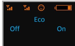
**NOTE:** the Eco mode status (activated/disabled) remains when switching the module off.
