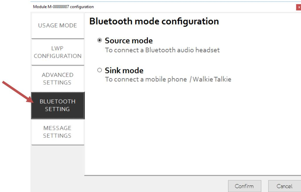
The new configured mode will be activated by confirming this menu then pressing « next » in the following window (see step 14 and 15)
