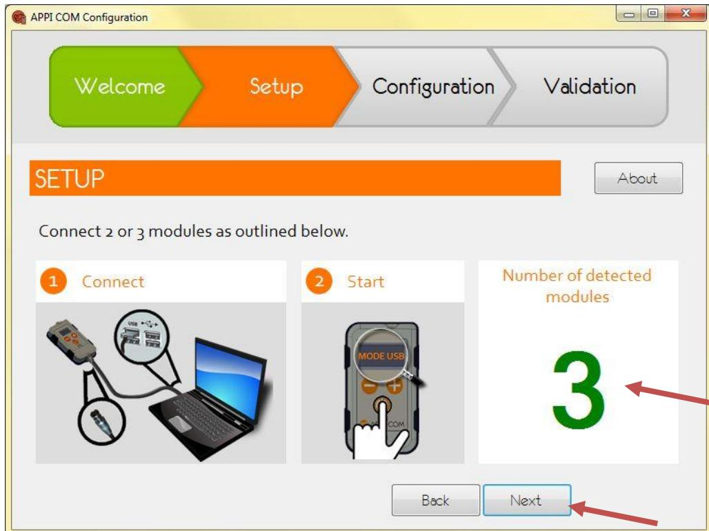
**NOTE:** « Next » would only be accessible when 2 or 3 modules are detected.
