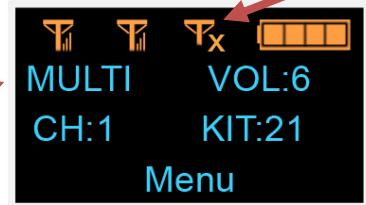
If no “**multiplex**” module communicates, the user can press his PTT and enter the conversation: his screen then indicates that he’s in the loop (smiley on the 3<sup>rd</sup> slot)
