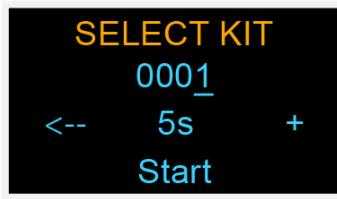
**The proposed kit to listen to is the last used on the selected channel** (in the example above, this is kit **1**). The user can, for 5 seconds (countdown), modify the kit to listen by using the keyboard buttons:
