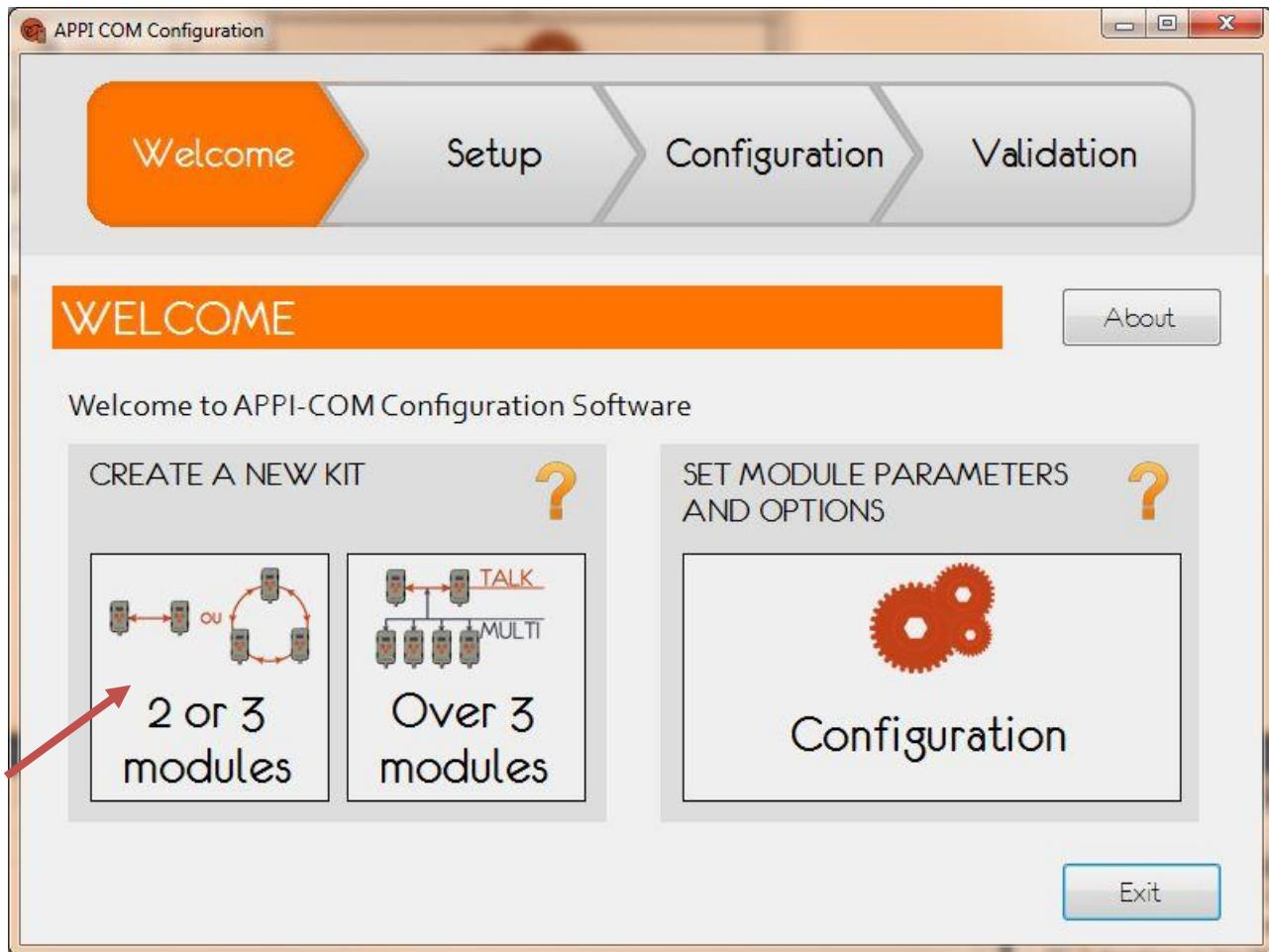
3. After clicking on “2 or 3 modules”, the software requests to connect the modules and indicates the number of detected modules.
