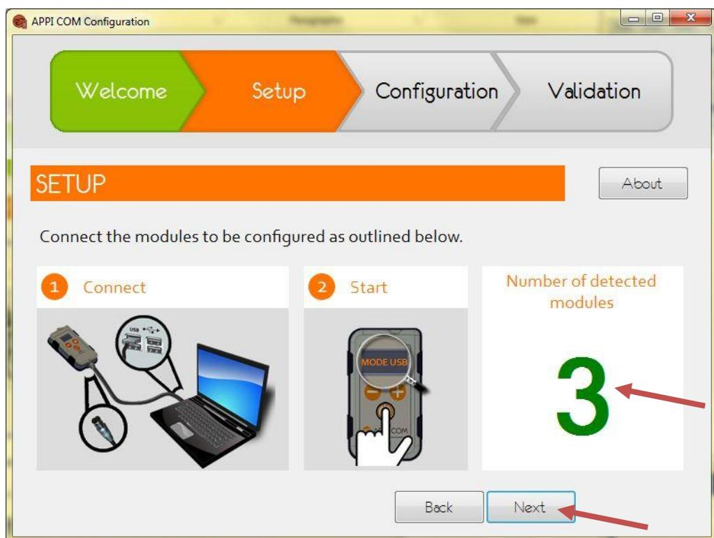
**NOTE:** the « Next» button is only accessible if 1, 2 or 3 modules are connected
