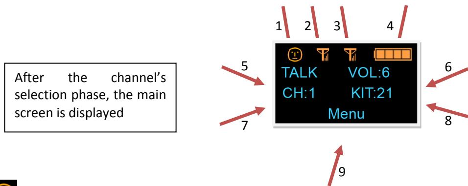
1. A « smiley » indicates the **module's Rank (1, 2 or 3) in the kit** as displayed on the screen with the arrows 1, 2 et 3 (here room 1 means rank 1)
