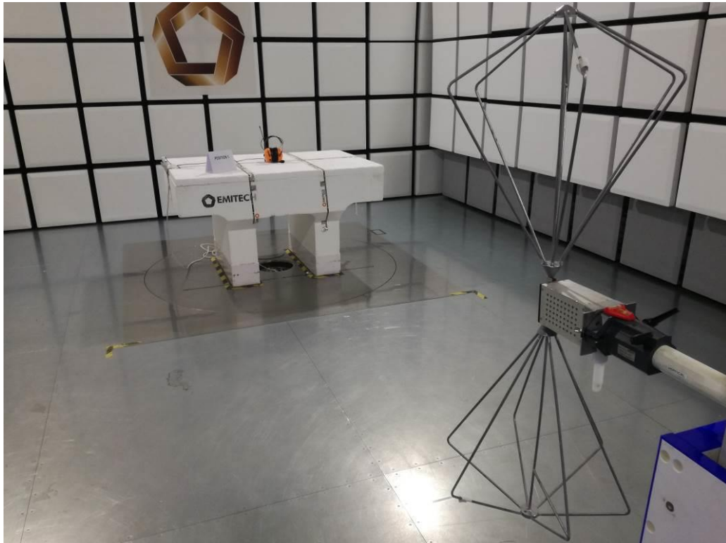
TEST SETUP PHOTO(S) – FOR FREQ < 200MHZ
