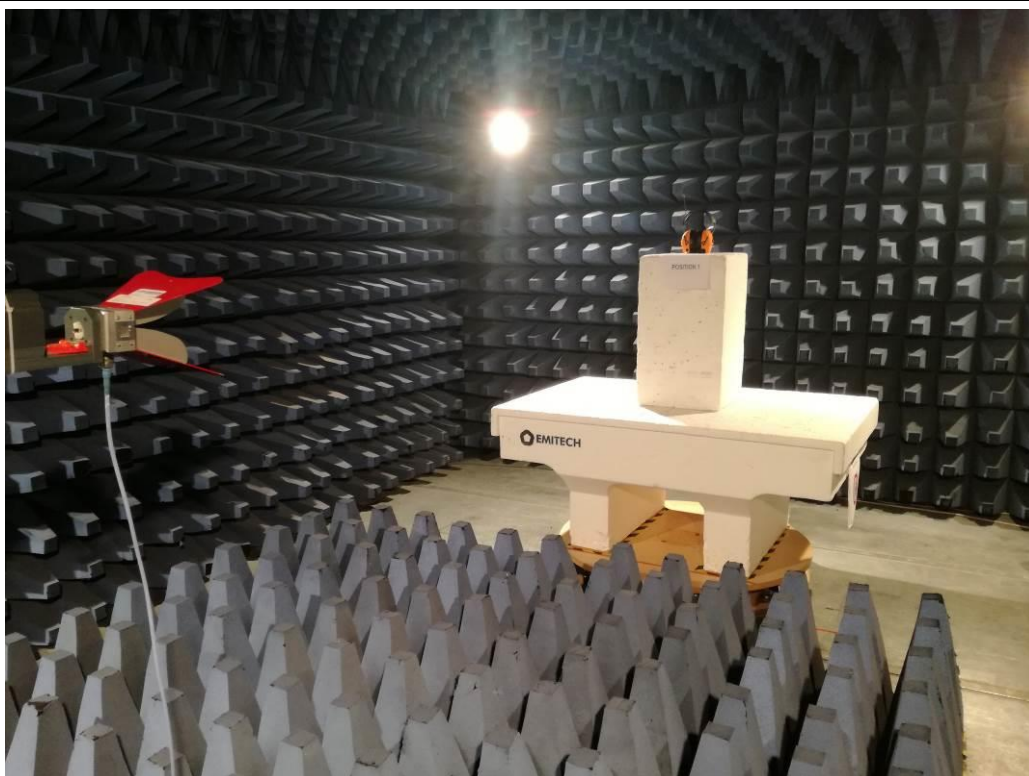
TEST SETUP PHOTO(S) – FOR \text{FREQ} > 1\text{GHz}
