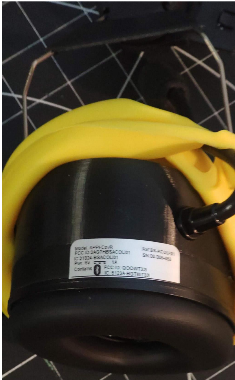
Figure 2. APPI-CovR Earmuffs Product Label position is under silicon IsoSkin.
