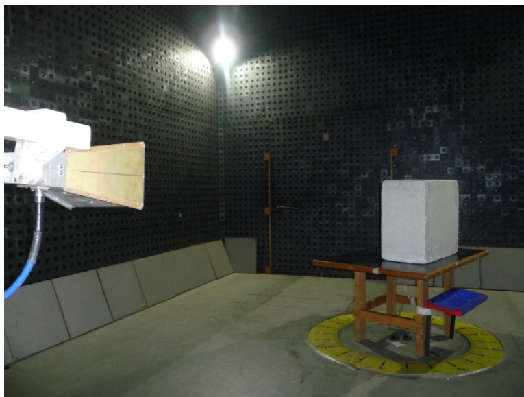
Photograph 8.1.3 Setup for radiated emission measurements above 1000 MHz
