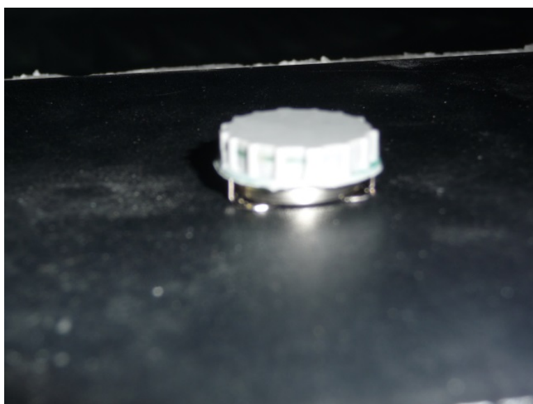
Photograph 8.1.2 Setup for radiated emission measurements, EUT in horizontal position
