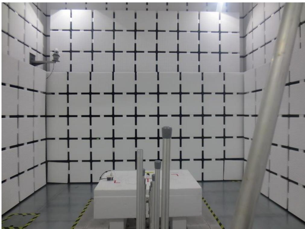
**Radiated Emissions Test Photos****Above 1 GHz**
