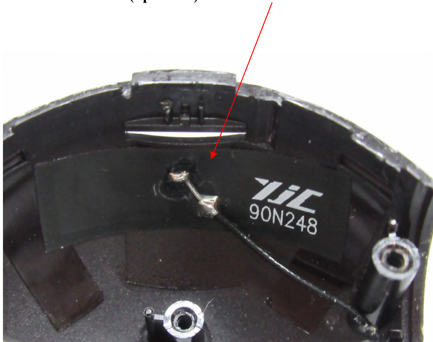
EUT (Speed 4S) – Wi-Fi Antenna View
