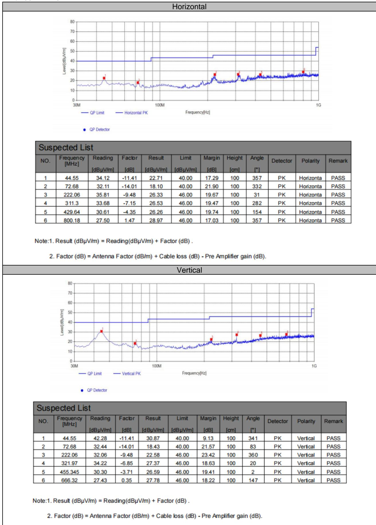
**For Greater than 1GHz****5150-5250MHz:****IEEE 802.11a (Worst Case)****802.11a Mode\_Channel 36\_5180 MHz**
