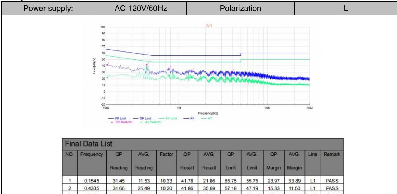
Note:1. Result (dB $\mu$ V) = Reading (dB $\mu$ V) + Factor (dB).
