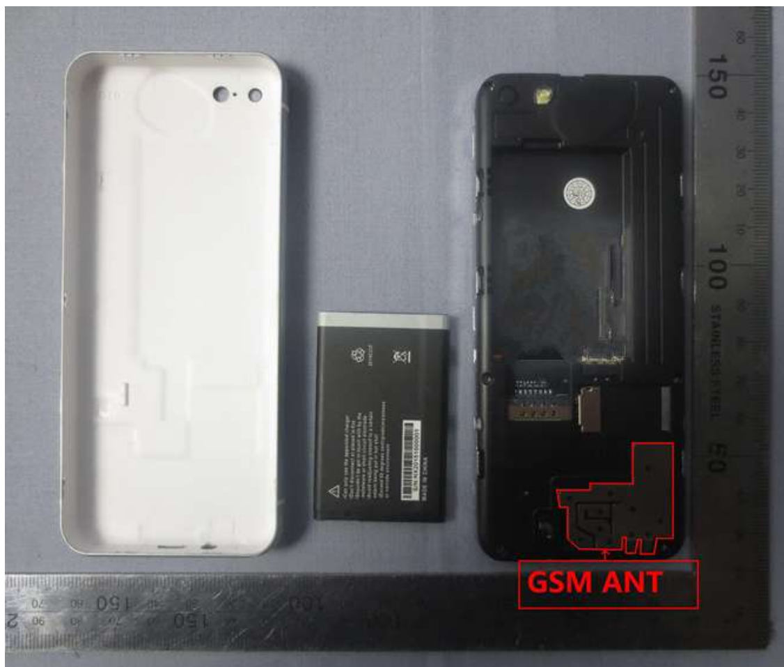
Fig.14.1 EUT Antenna Locations
