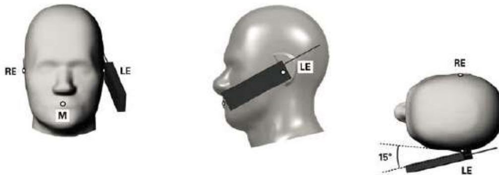
Fig.11.4 Illustration for Tilted Position
