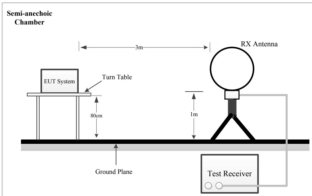
The test was performed in the 3-meter chamber test site, using the setup accordance with the ANSI C63.10-2013.
