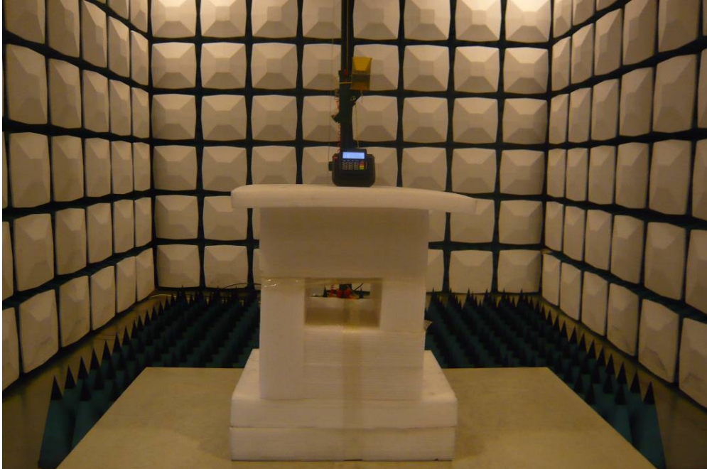
Radiated Emission View (Above 1GHz)
