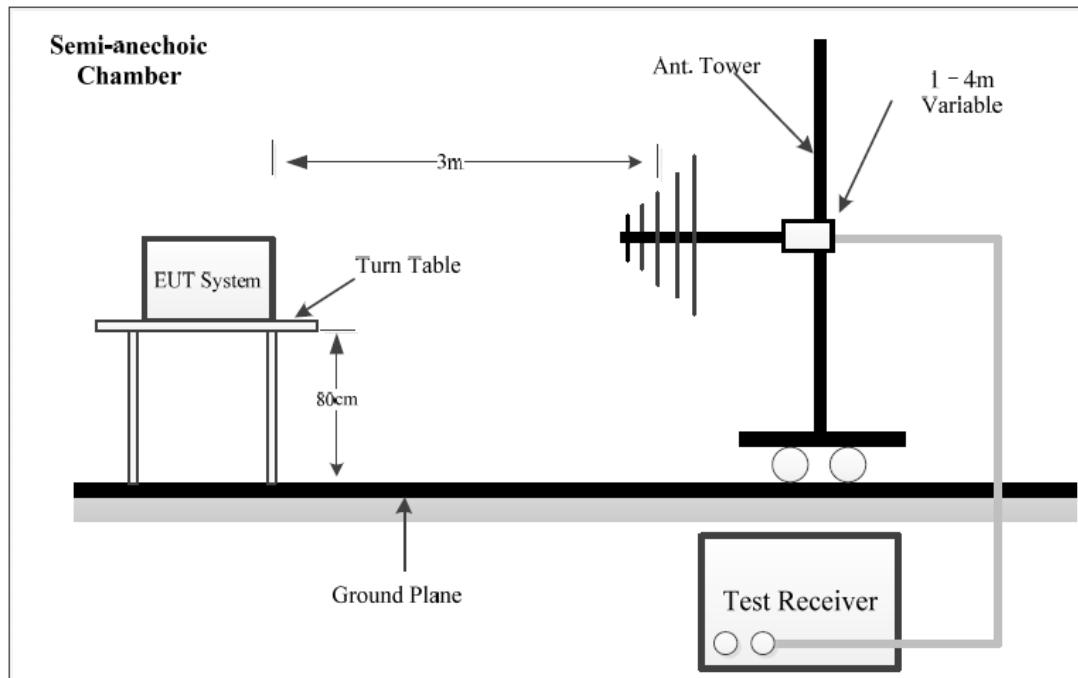
The radiated emission tests using the setup accordance with the ANSI C63.10-2013. The spacing between the peripherals was 10 cm.
